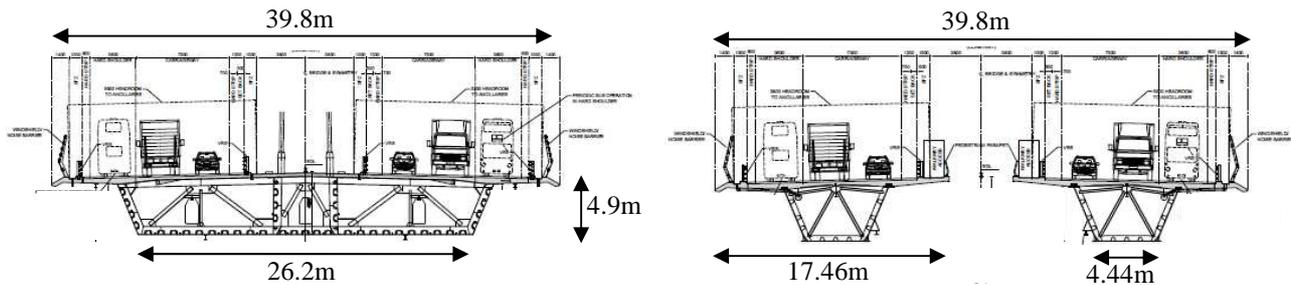
Typical Main Cable Stayed Span Cross Section
