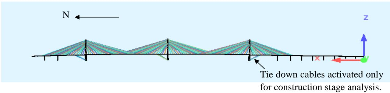
**Picture 4 Fleshed Bridge Global Model in Elevation**
