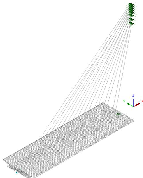
**Picture 8 View of Typical Semi Global Model**
