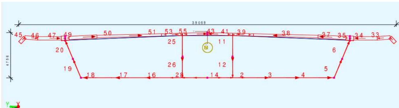
**Picture 5 Cable Stayed Bridge Cross Section (Grafix)**
