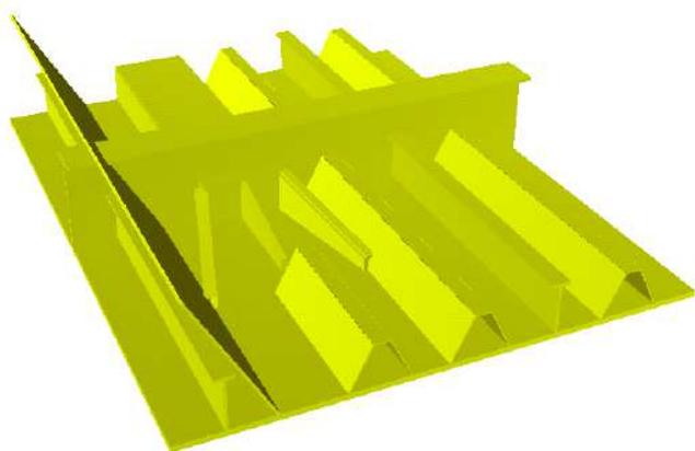
**Picture 9 Sub-model of Steelwork Details on Bottom Plate of Deck**
