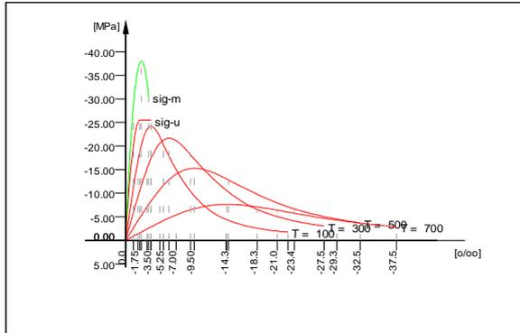
**Fig 1: Stress-Strain relationship for concrete under compression under elevated temperatures according to EC 2**
