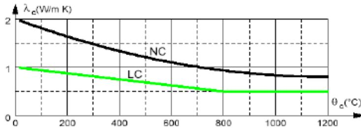
**Fig 5 : Thermal conductivity of normal concrete and light concrete vs. Temperature**
