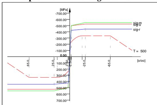
**Fig 2 Stress-Strain relationship for reinforcing steel at elevated temperatures according to EC 2**
