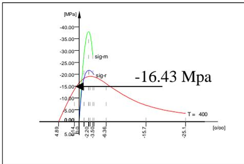
Fig 11: Material law with SHIFT for concrete at T=400 ° C
