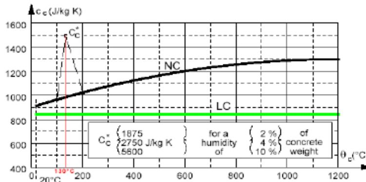
**Fig 6 : Specific heat capacity of concrete**
