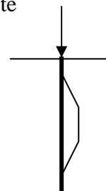
Under elevated temperatures for a column fixed at the top and bottom by a reinforced concrete slab, it can be assumed that the ends are fixed against rotation.
