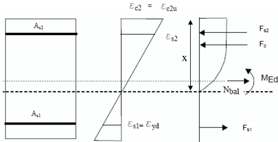
**Fig 9: Internal resistance and bearing moment for the assumed strain plane.**
