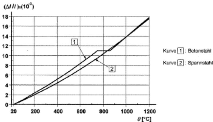
Fig3 Thermal expansion of reinforcing and pre-stressing steels according to EC 2
