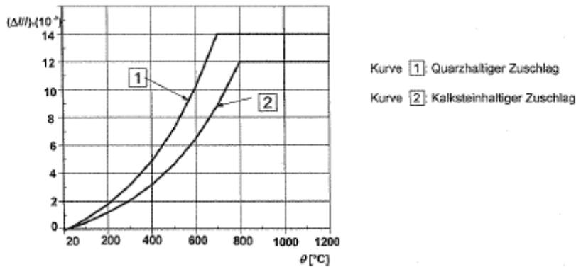
Fig 3: Thermal expansion of concrete according to EC 2
