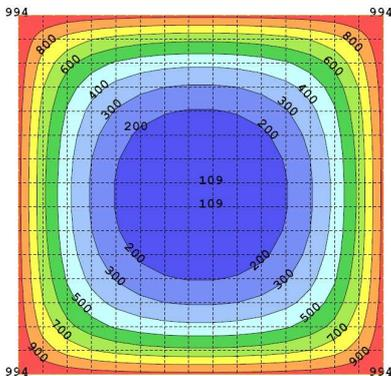
Fig 15: Temperature zones for T= 90 min acc. To ISO 834 Time – temperature curve, Section size 30x30 cm
