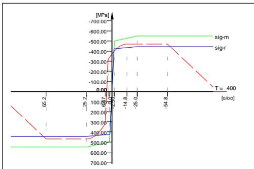
Fig 12: Material law with SHIFT for reinforcing steel at T=400 ° C
