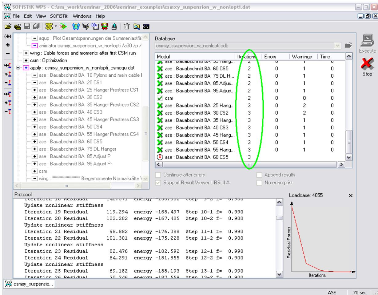
Figure 6: SOFiSTiK WPS during optimization iteration
