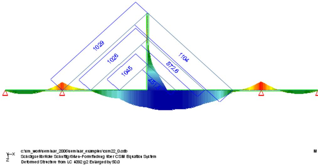
Figure 3: Bending moments and cable forces w/o CSM Equation system optimization
