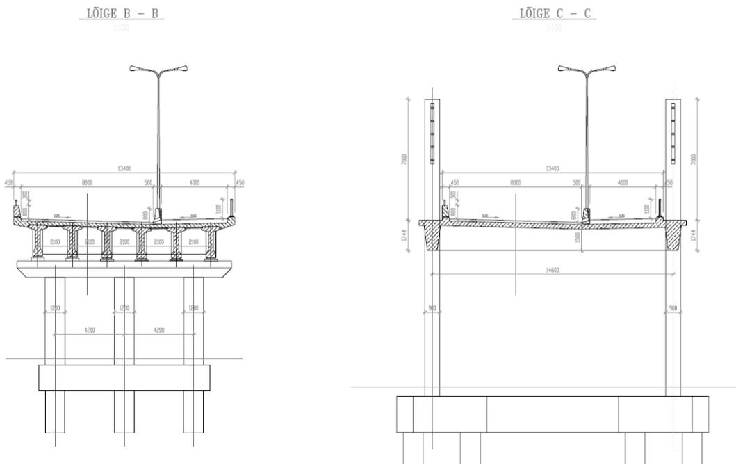
**Figure 16: Cross-sections of approach and main span**
