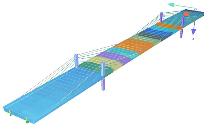
**Figure 15: Structural model of the main bridge**
