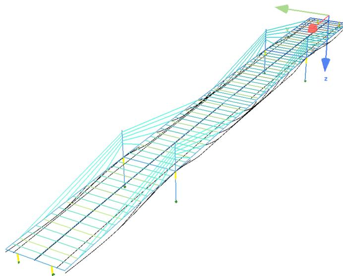
**Figure 18: Pre-stressing layout in main girders**
