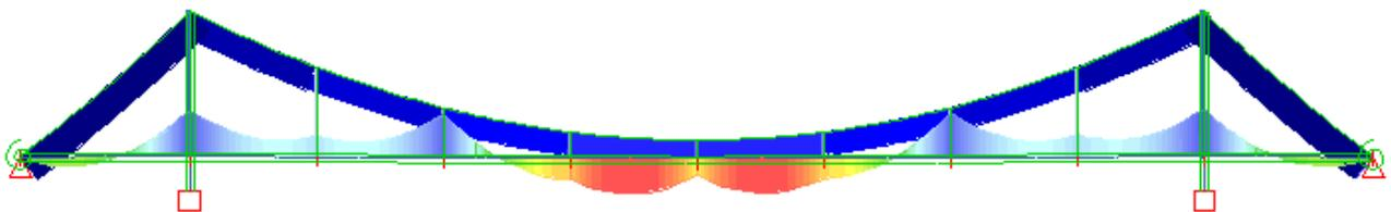
**Figure 9: Beam and cable forces after CSM Equation system optimization**
