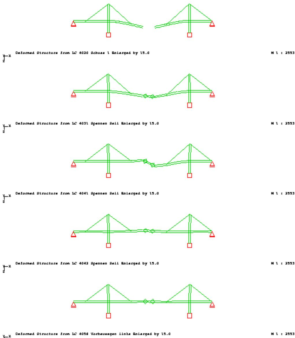
Figure 12: Construction sequence of csm23\_cable\_stayed\_opti\_displacements.dat
