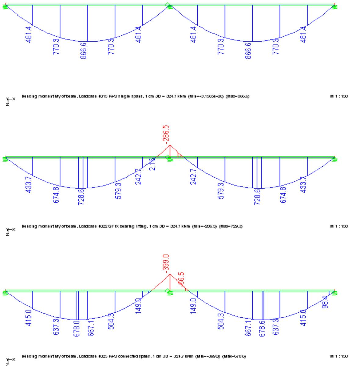
**Figure 13: Bending moments of a precast girder system; Hogging moment limited to 400kNm due to CSR with the CSM Equation system**
