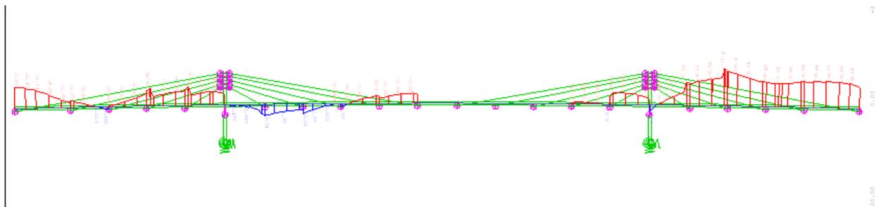
**Figure 22: Stresses in main girder at Stage 9**
