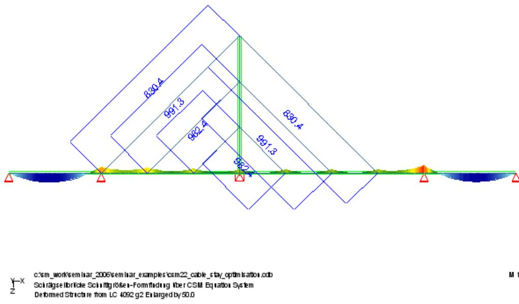
Figure 4: Bending moments and cable forces with CSM Equation system optimization
