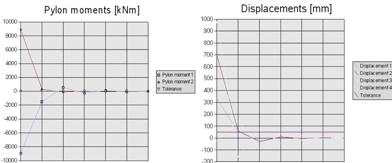
Figure 7: Convergence behaviour of the objectives during optimization (7 Iterations)
