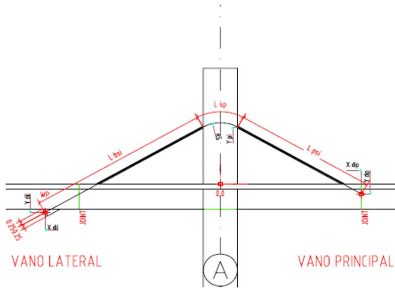
Figure 19: AutoCAD detail of cable anchorages
