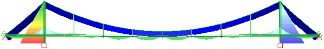
**Figure 8: Beam and cable forces on the built-in-one system**
