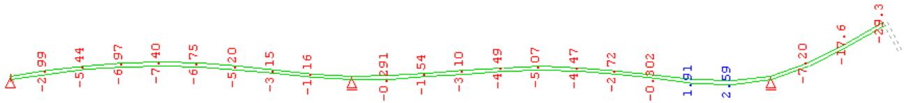
**Figure 1: Precamber of formwork (nodal values in mm)**
