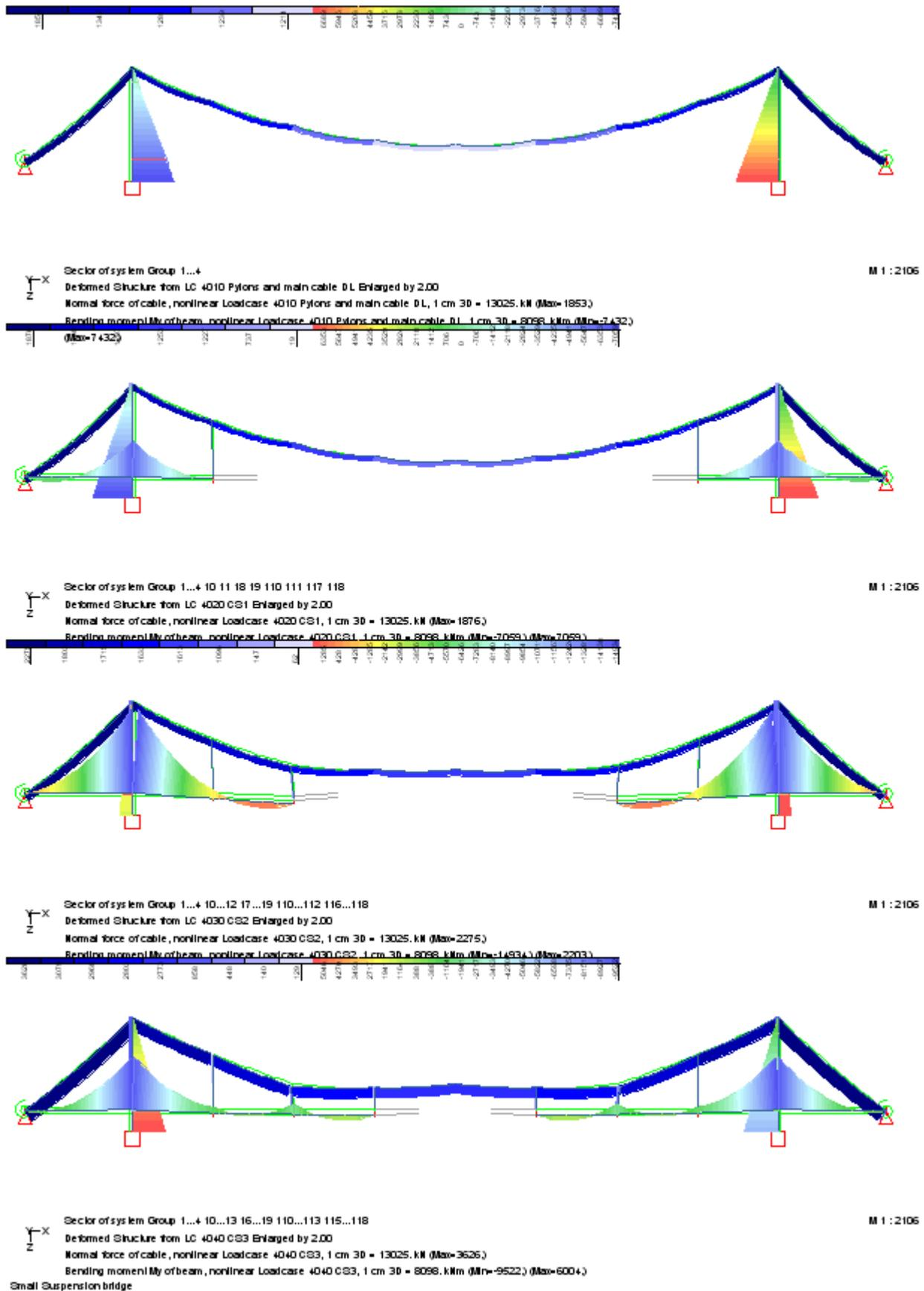
Figure 10: Optimized construction stages 1-4 of the suspension bridge
